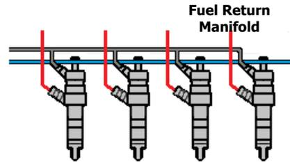
Fuel return manifold carries away fuel that was not injected for combustion
