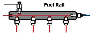
Acts as snubber to dampen supply pump pressure pulses
